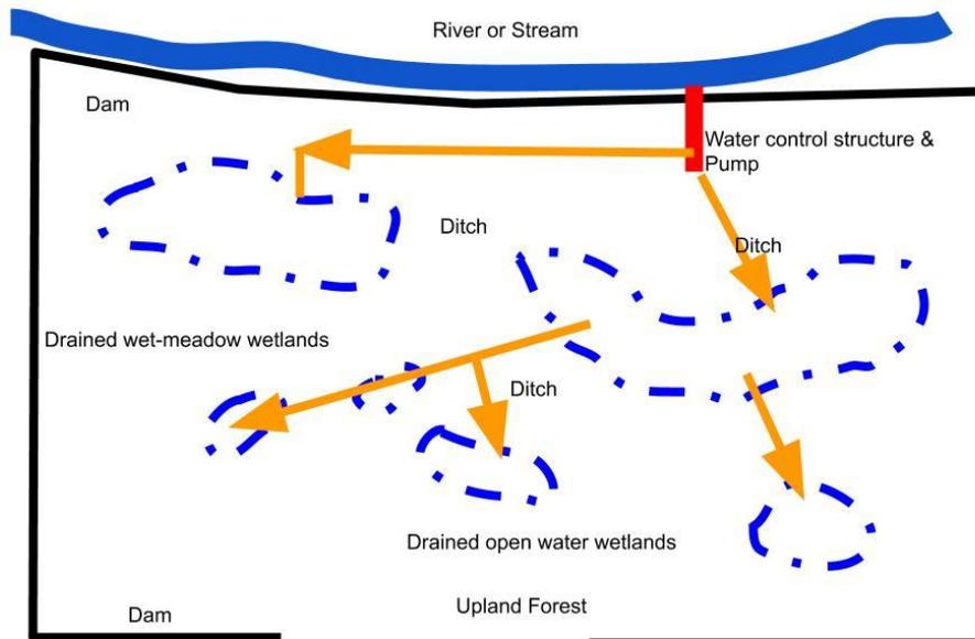
This impoundment is designed to be filled by pushing water uphill. Water soon leaves the natural wetlands when pumping ends.
