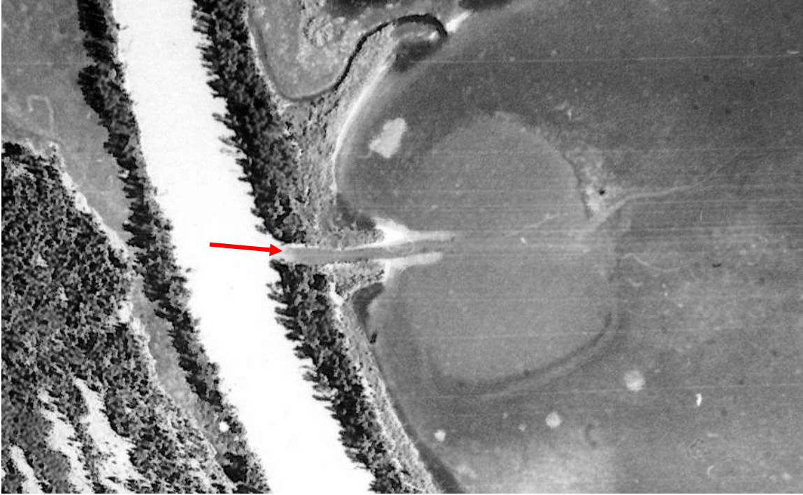
This 1958 aerial photograph clearly shows water flowing into Six Mile Slough from the Kootenay River. A channel had been dug between the deep-water pond, now in wetland compartment 3, and the Kootenay River. The deep pond may have been dug to provide water for livestock, and to act as a sump for draining Six Mile Slough.
